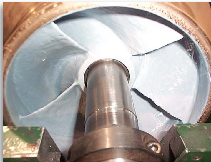
Impeller with Belzona Coating
